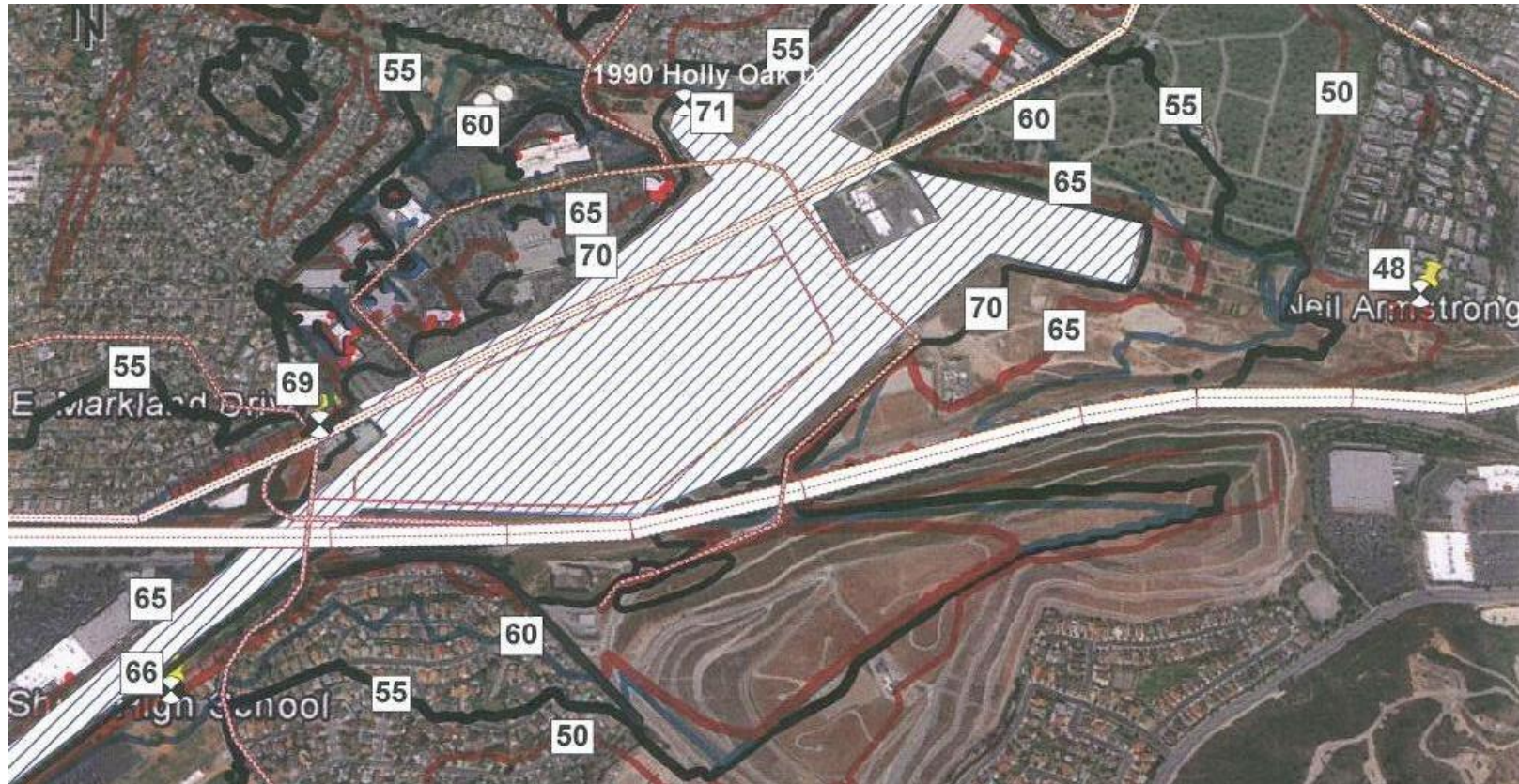
Figure 4-1 Construction Noise Contours – L_{eq}(8\text{-hr}) , dBA
