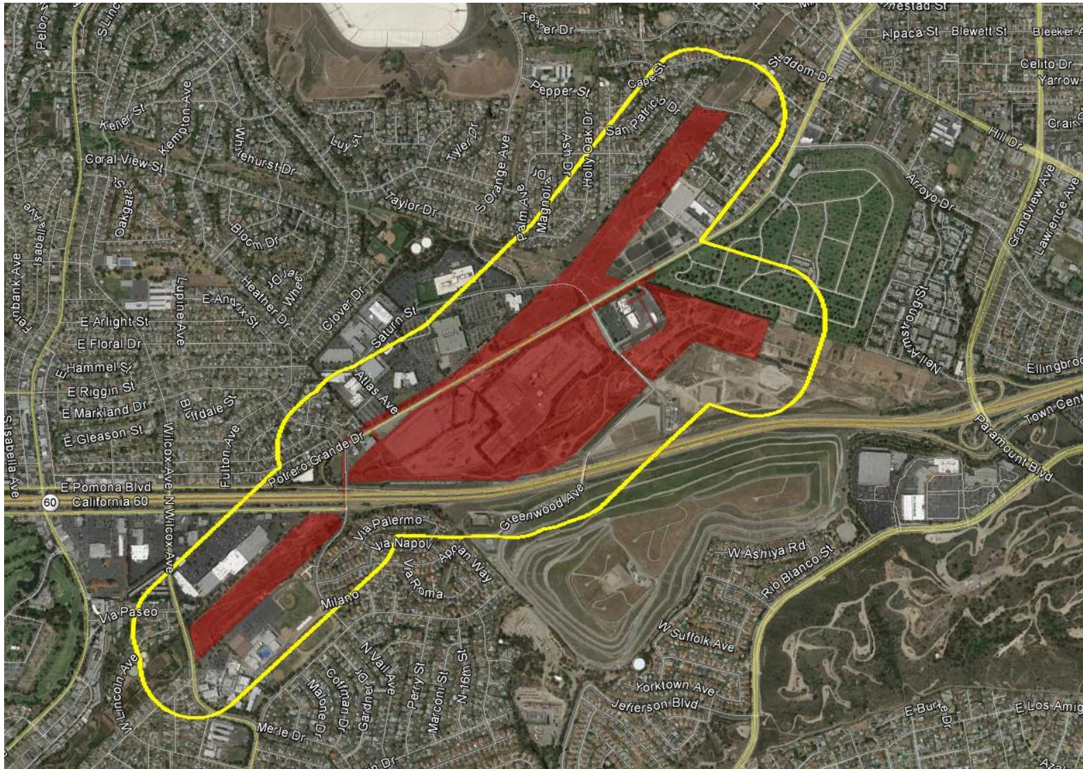
Figure 4-2 80 dBA L_{eq}(8\text{-hr}) Contour For Helicopter Use in ROW
